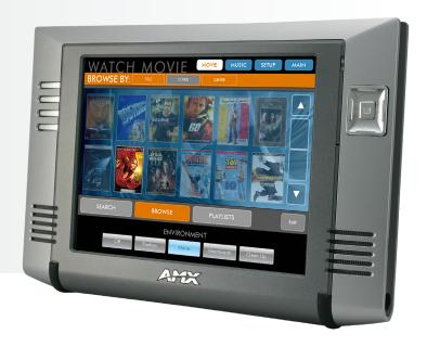
The MVP-8400 is a clean, seamless, unobtrusive touch panel that combines Wall/Flush Mount flexibility, table top functionality and wireless mobility that gives users the ability to take control from anywhere, at any time. A fully compatible standard 802.11 Wi-Fi Card provides additional control features and eliminates the inconvenience of installing and using cables. Additionally both 38KHz and 455KHz 1-way IR are also built in.
